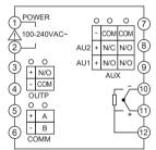
Note 1: Dimension D61 instruments does not support 0~1V and above linear voltage input. Instead, 0~1V signal can be converted to 0~100mV by external voltage divider while 4~20mA can be converted to 20~100mV by connecting a 5 ohm resistor in parallel, then be inputted from terminals 11+ and 10-.
