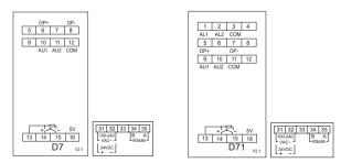
Note 1: Input 0~5V/1~5V input from 16+, 15-. 100mV below input from 14+, 15-4~20mA with 250ohm shunt resistor converted to 1~5V, input from 16+, 15-
